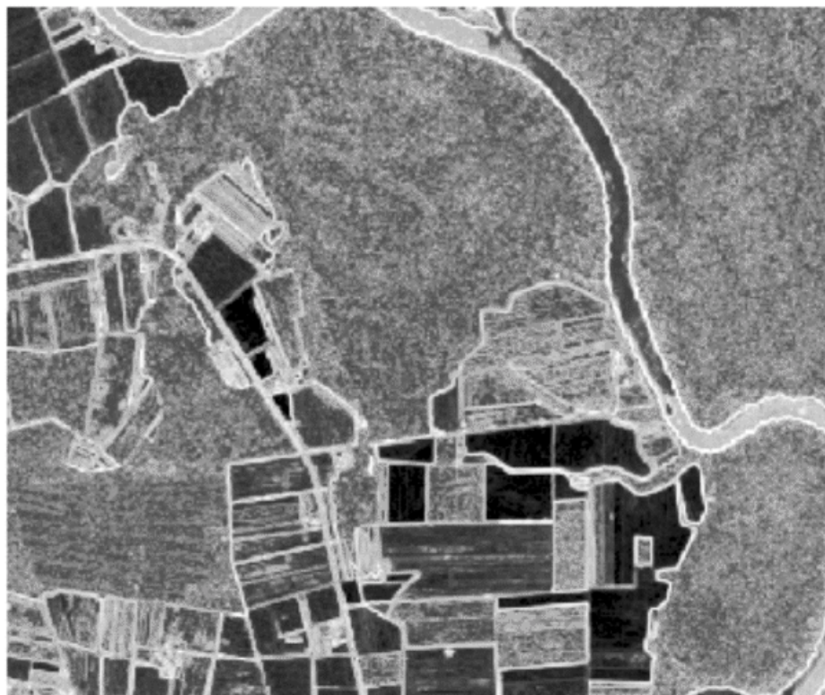
Figure 2. Example of the application of average spectral angle auto-correlogram operator to an agricultural scene. Wavelength range 0.5 - 1.1 micrometers.
