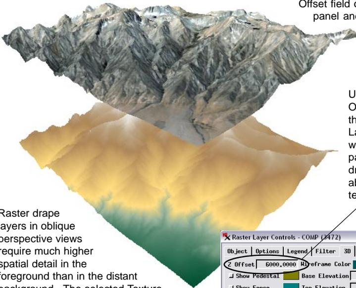
Use the Z Offset field on the Raster Layer Controls window's 3D panel to float a drape layer above the terrain.
