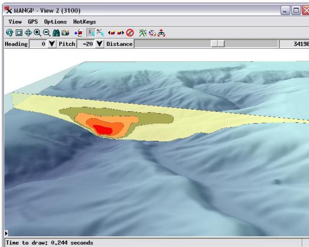
You can set up a raster or a 2D vector object to display as a manifold using the Georeference process. Simply assign 3D control points using the 3D Piecewise Affine model. Refer to various Technical Guides at [microimages.com](http://microimages.com) for more information.
