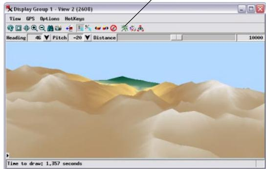
The 3D perspective window shows either wireframe or solid renderings of the spatial data.
