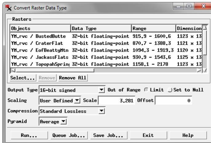
Convert Raster Data Type window. The input elevation rasters have floating-point values in meters; these values are being rescaled to integer feet in the 16-bit signed data type using a User Defined scale factor. The illustration below shows a display of the source and result for one of the elevation rasters with a DataTip showing the source and output values for one raster cell location.
