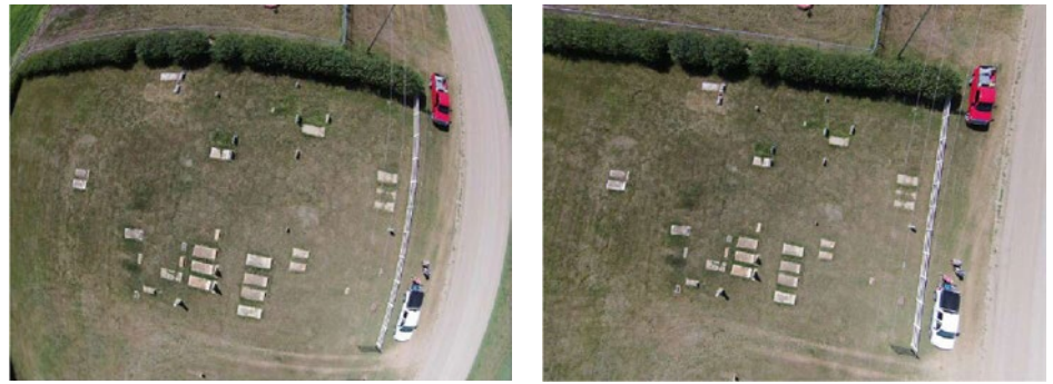
Left: UAV camera color image with severe barrel distortion from a very wide angle lens. Right: same image after correction in TNTmips for Geometric Distortion.
