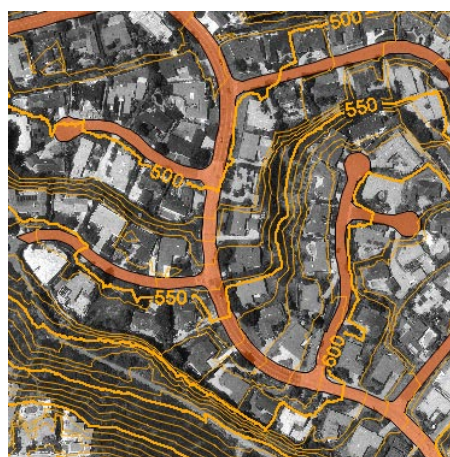
Topographic contours (orange, with 10-foot contour interval) overlaid on portion of orthoimage (0.15-meter cell size), both obtained from County of San Diego. Street overlay (red fill) traced from same orthoimage for testing. Area has 200 feet (60 meters) of relief from lower right to upper left; width of area is 440 m.
