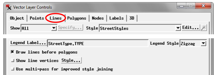
Element-specific controls on the Lines tabbed panel
