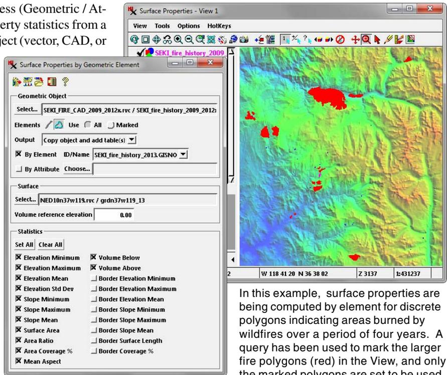
In this example, surface properties are being computed by element for discrete polygons indicating areas burned by wildfires over a period of four years. A query has been used to mark the larger fire polygons (red) in the View, and only the marked polygons are set to be used.
