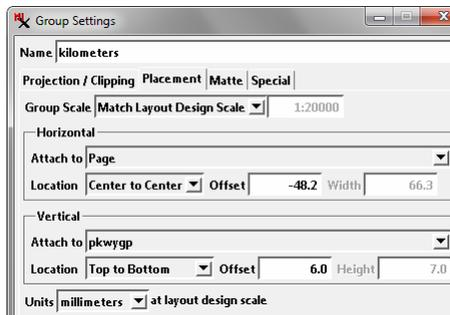
The *kilometers* scale bar shown below with the Layout Placement tool has its center attached horizontally to the page center (vertical dashed black line) and its top attached vertically to the map group (*pkwygp*) above it.
