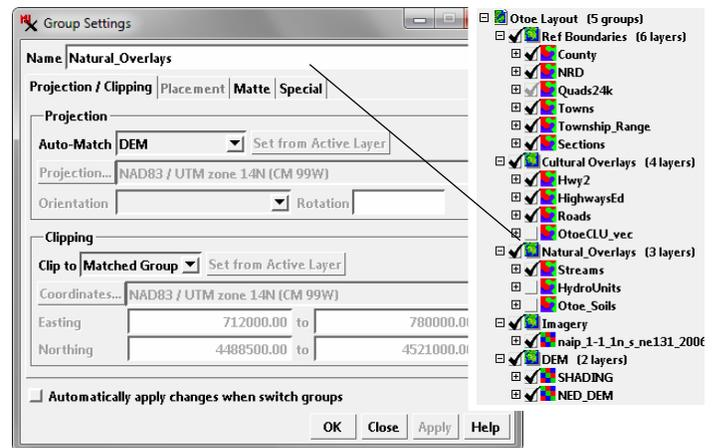
Projection / Clipping panel in the Group Settings window for a group in a display layout for an electronic atlas. This group's coordinate reference system has been set to automatically match that of the bottom group (DEM) in the layout. Its display extents have also been clipped to those of the matched group.
