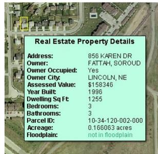
In these illustrations, a Display Control Script (DTbackgroundByAttribute.sml) is used to create the heading for the DataTip and to change the background color depending on the floodplain status of the property at the current cursor location.
