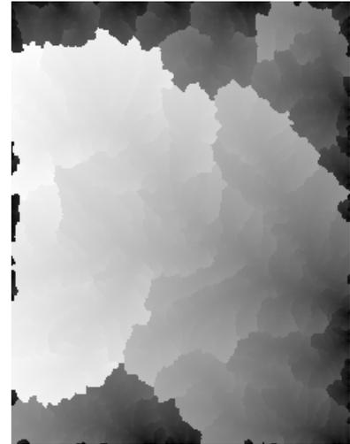
⑥ Downstream flow distance raster. Cell value equals the downstream flow distance from the current cell to the watershed outlet.
