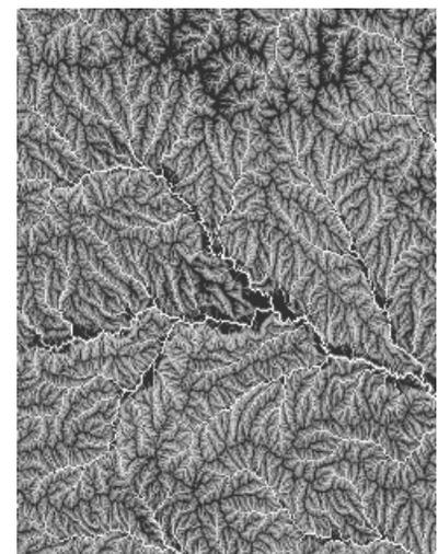
③ Length-Slope raster computed from specific catchment area and slope. High values occur along major flowpaths due to high values of specific catchment area.
