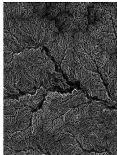
② Slope raster. Brighter tones indicate higher slopes. The lowest slope values are on valley floors and ridge tops.
