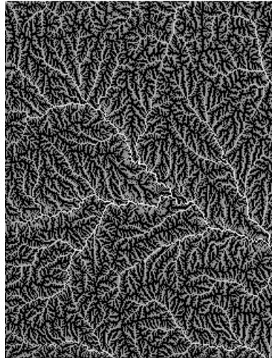
⑤ Maximum upstream flow distance raster. Cell value equals the longest flow distance from the upstream watershed boundary to that cell.
