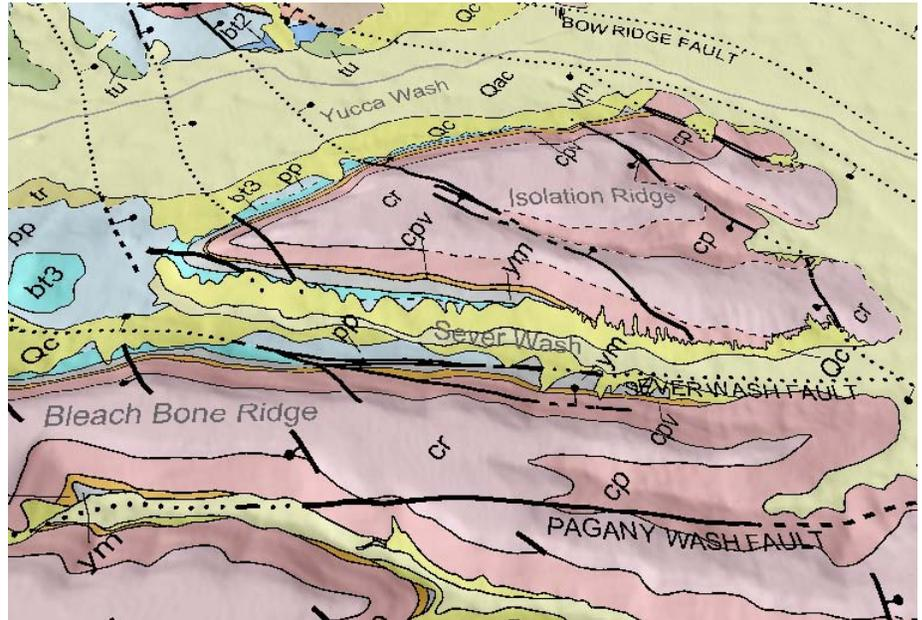
This 3D rendering of geologic map data combines a shaded-relief raster layer with six vector layers. The layer with geologic map polygons includes polygon labels with the rock unit symbol, some of which are drawn outside their polygon with leader lines. The layer with faults (bold lines) includes line labels with the names of the faults. Another layer provides text labels for topographic features.
