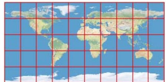
Left, table showing range of possible pre-rendered, fixed zoom levels in a NASA World Wind tileset. World Wind uses an equirectangular (Plate Carree) earth model and a tile size of 512 pixels. Its lowest zoom level is a 5 x 10 array of tiles with each tile covering 36 degrees of latitude and longitude, as shown in the illustration above. Each subsequent zoom level doubles the number of tiles in both directions, as in Google Maps and Bing Maps.
