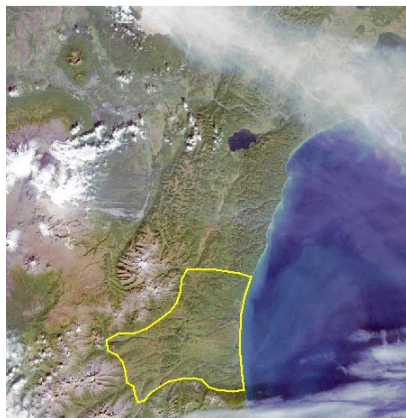
Extract of a Landsat scene displayed using bands 3-2-1 to produce a natural color display. The scene includes clouds, snow cover in high altitude areas, a volcanic eruption cloud (top), and ocean. The yellow polygon is a region outlining a vegetated lowland target area to be enhanced.
