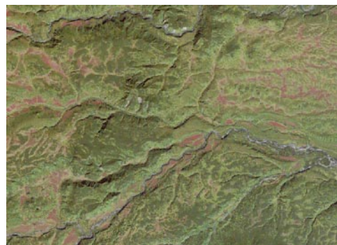
Zoomed-in view of part of the lowland area with normalized contrast based on the histograms for the entire image. This display of the lowland has poor contrast and color due to the influence of the bright and dark scene areas.
