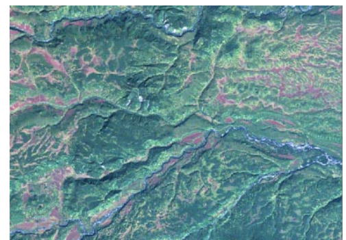
View of the lowland area with Linear contrast designed using local histograms for the lowland region. This display of the lowland area has better contrast and color than the view with global normalized contrast.
