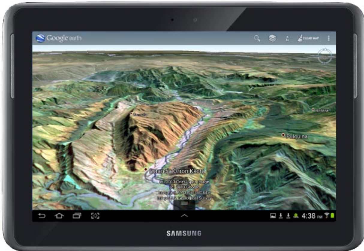
Google Earth Android app showing a custom tileset created in TNTmips from three bands of an ASTER satellite image of an area in Bolivia (middle infrared, near infrared, and green bands as red, green, and blue, respectively).
