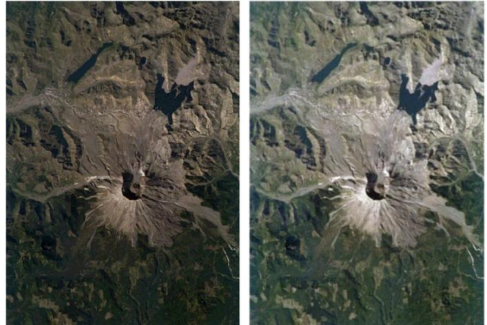
Display of RGB image with no enhancement (left) and with contrast-enhancement (right) for the red, green, and blue components.
