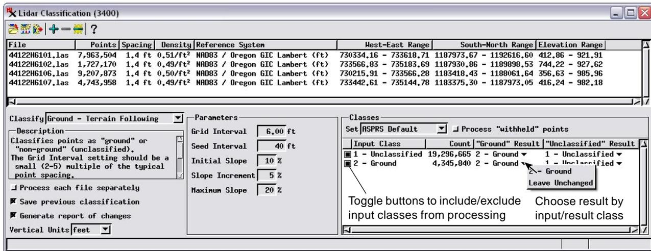
The Classes list in the Lidar Classification window allows you to choose which classes of points in the input files to process, and also lists the potential result classes produced by the selected classifier (such as Ground and Unclassified for the Ground classifier shown). For each combination of input class and result class, press the small arrow icon to open a menu to choose whether to accept the classifier result or leave the point class unchanged.
