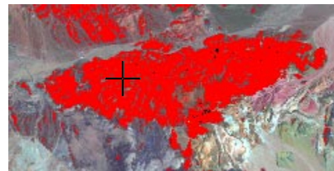
Feature Mapping view after additional sample cells were added in darker basalt areas and Classify procedure was run again to create an expanded prototype set. A number of spatially separated areas have been included within the prototype set.
