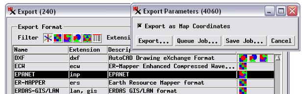
INP files do not include EPANET simulation results; these can be saved in EPANET in other text and binary file formats. Thus there is no need to re-import the network to TNTmips after running an EPANET simulation.
