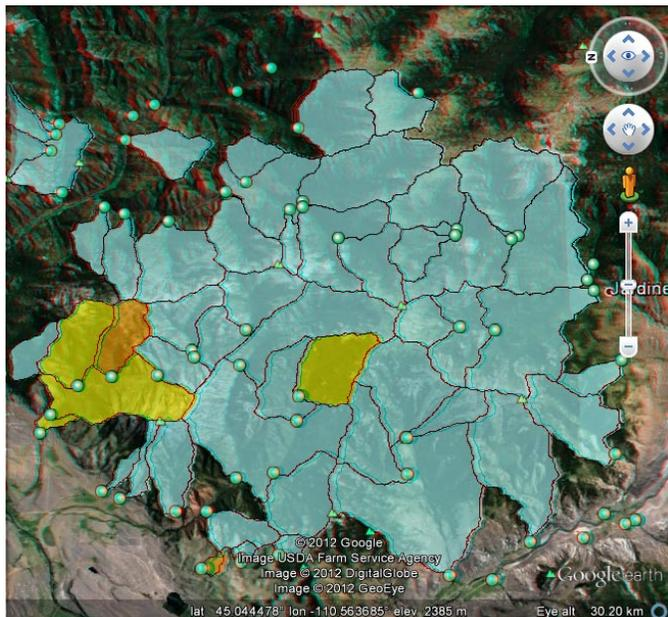
TriDef Google Earth anaglyph stereo view of KML geometric tilesets created in TNTmips. Point symbols are locations of stream sediment samples with geochemical analyses. Polygons are stream catchments delineated by the TNTmips Watershed process, with polygon fills indicating relative copper content of sediment, with yellow indicating highest values.
