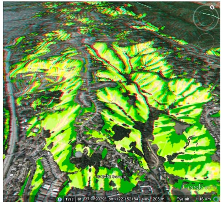
TriDef Google Earth anaglyph stereo view of a Google Earth standard web (raster) tileset rendered from a theme-mapped raster object in TNTmips. The tileset depicts relative hazard from landslides in the Oakland-Piedmont area of California; yellow color indicates highest hazard.
