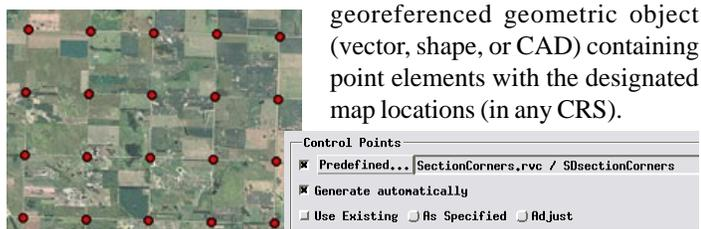
Display of section corner points (red symbols) from the US Public Lands Survey System, many of which correspond to section-line road intersections in much of the midwestern United States. A geometric object containing these corner points optionally could be used to designate predefined candidate locations for recognizable control points in autoregistering images from this region.
