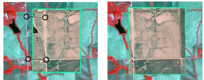
Close-ups of View-In-View overlays of the original SPOT scene (outside green box) and the reference orthoimage (inside green box). Left illustration shows the SPOT scene with nominal georeference; linked black circles indicate corresponding ground features offset by about 300 meters. Right illustration shows excellent registration of the SPOT scene with the control points generated by auto-register.
