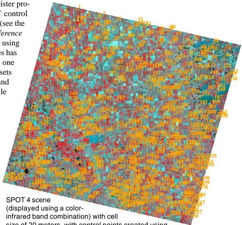
SPOT 4 scene (displayed using a color-infrared band combination) with cell size of 20 meters, with control points created using the Auto-Register procedure in the sample SML script. The reference image is the South Dakota 2010 GM\_BM web tileset hosted at microimages.com (derived from NAIP natural-color county orthoimages).
