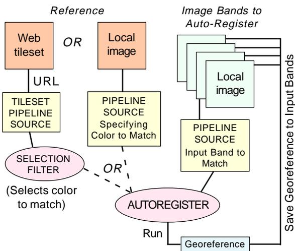
Although the auto-register operation in SML utilizes image pipeline structures, it is not a complete pipeline operation, as no new "target" image is created, only georeference information.
