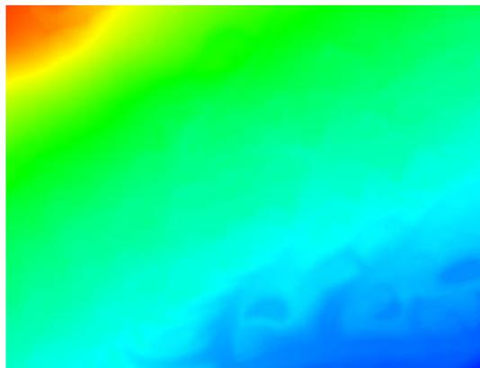
Virtual surface for the sample area constructed using only bare earth points and displayed using the Elevation terrain option with the color spread shown in the Elevation Color interface illustration to the right. The elevation colors highlight the general southeast slope of the bare earth surface.
