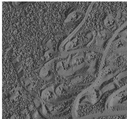
Shaded virtual surfaces for the western portion of the sample area using all LIDAR point classes, including buildings and vegetation. The surface on the left was constructed using the Single and Last option from the Returns menu. In the forested area, the last of multiple returns reaches deeper into the tree canopy and in places reaches the ground. The surface on the right was constructed using the Single and First return option, and thus models more of the tree canopy in the forested area.
