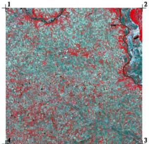
Input Image: SPOT 5 image (4 bands) acquired during the 2009 growing season over an area in southeast Nebraska, displayed with three bands to produce a colorinfrared image. The image is 6,000 columns by 6000 lines with a cell size of 10.2 meters. The four corner control points produced from the georeference supplied with the image yield RMS residuals X = 11.46 cells, Y = 1.53 cells, XY = 11.46 cells using the Affine model.
