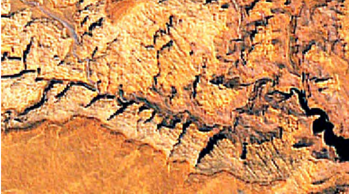
using a custom sharpening filter (filter kernel shown in the illustration above) designed to enhance edges with a northwest trend
