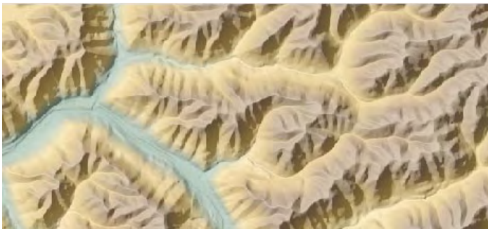
Left, an elevation raster with color palette displayed with partial transparency over a shading raster to provide a color shaded-relief display. Right, the same raster layers are displayed with a
