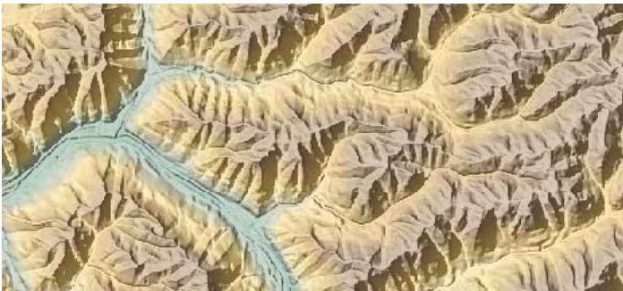
5 x 5 Volterra/Unsharp sharpening filter applied only to the shading raster layer, producing a crisper image of the terrain.
