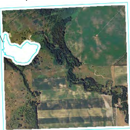
Result of Raster Extract with the area selected by region and buffered inside satisfies both inside section roads and outside lake area in a single pass. Region is shown along with extracted raster result above.
