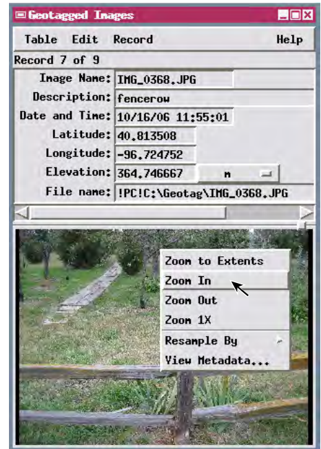
A Single Record View of a geotagged image table (above) automatically shows the image for the current record in the bottom part of the same window. Right-click on the image to pop in a menu with zoom and other options. This example shows a table with linked (rather than embedded) images.
