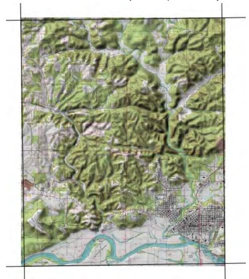
Above, one shaded DRG quadrangle file. The files were processed by UAM SAL so that the edge portion of each raster outside the quadrangle boundary (overlay of black lines) includes data from the adjacent quadrangles, leaving no blank edge cells. This processing allowed assembly of a seamless multifile raster with no blank cells along the seams between adjacent quadrangles.
