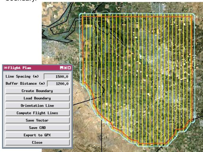
Pressing the Compute Flight Lines button creates the buffer zone (cyan in this illustration) around the boundary and the set of flight lines (yellow). You can then save the flight lines, boundary, and buffer boundary as separate vector or CAD objects, and export the flight lines to a GPS Exchange (GPX) file for use in navigation.
