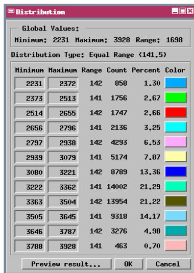
Pressing the Run button on the Raster Intervals window opens the Distribution window, which lists the value ranges initially determined by the script and statistical information about them. You can use this dialog to customize the ranges by editing the minimum or maximum values; adjacent ranges are automatically adjusted in response to your changes.
