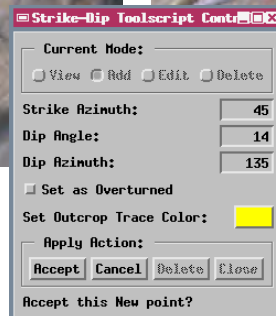
The Tool Script’s control window provides View, Add, Edit, and Delete modes.
