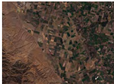
SRFI Option 2: Scaled reflectance corrected for atmospheric path reflectance. Haze is removed, but remaining atmospheric attenuation effects make images too dark and too red.
