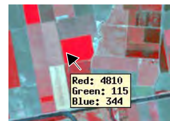
SRFI Option 3: Scaled reflectance of Earth surface materials with all atmospheric effects (path reflectance and atmospheric attenuation) removed. Remaining brightness variations due to varying slope angles and directions in hilly areas can be corrected using the TERCOR geospatial script (see the color plate entitled Scripts by Jack: Correct for Terrain Induced Radiance Effects ).
