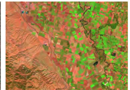
SRFI Option 2: Scaled reflectance corrected for atmospheric path reflectance. Haze is removed, but remaining atmospheric attenuation effects make images too dark and too red.
