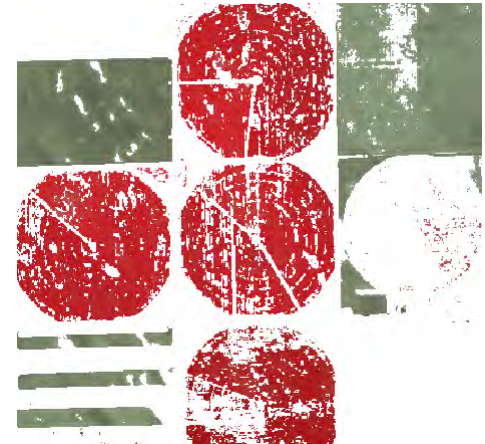
Bands processed with the DIAG script. Colored cells indicate dense green vegetation and bare soil. White areas are cells that have been set to null by DIAG-script processing.
