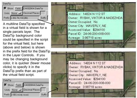
script for a virtual field that provides the DataTip for a layer. Colors can be specified by name if the color is in the color lookup file used by the TNT products (rgb.txt) or by percentage of each color component in RGB order. The illustrations at the left show the DataTip set on the Polygon tabbed panel of the Vector Layer Controls window for the parcel outline vector object described on the color plate entitled *Property Viewer Atlas for Lincoln, NE*.
