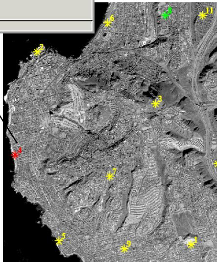
Control Points: Projected to Orthorectified Image
