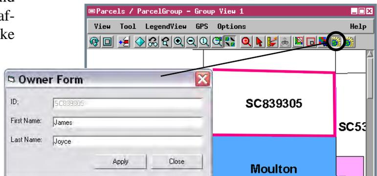
Modeless Visual Basic dialog “Owner Form” (in the imported class VBForm) that is launched by the ParcelToolModeless tool script. After the names are filled in, pressing the Apply button calls an `OnApply()` function in the tool script that reads the name fields from the VBForm class and updates the ParcelInfo database table and the TNT View window.
