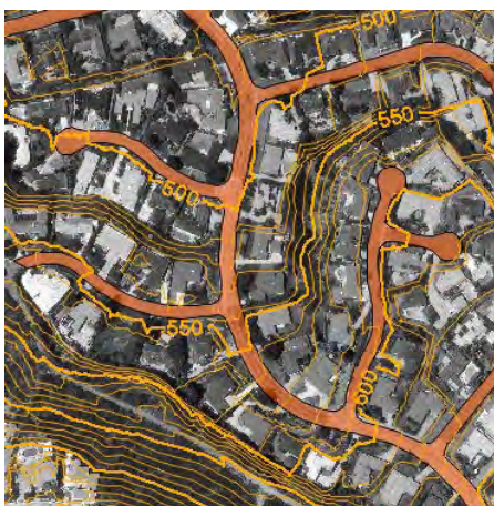
Topographic contours (yellow, shown with 10-foot contour interval) overlaid on portion of orthoimage (0.15-meter cell size), both obtained from County of San Diego. Street overlay (orange) traced from same orthoimage for testing. Area has 200 feet (60 meters) of relief from lower right to upper left; width of area is 440 m.
