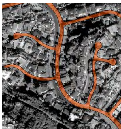
Street vector overlaid on portion of the IKONOS panchromatic image georeferenced with GPS points, prior to RPC orthorectification. Significant misregistration of the street overlay results from internal image distortion in the unrectified image due to local terrain relief.
