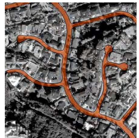
Street vector overlaid on IKONOS pan image after RPC orthorectification. Rectification successfully removed terrain relief effects from the image, so there is now excellent registration with the planimetrically-correct street overlay.
