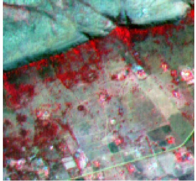
Same image area after the Forward FFT (Fast Fourier Transform) and Destripe procedures were run on the individual bands. Striping has been completely suppressed with no blurring or degradation of ground features.
