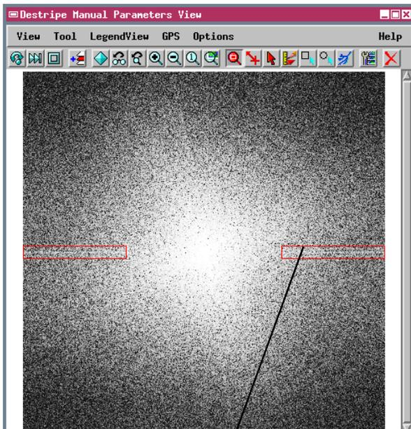
The Manual Destripping mode was used to process the ASTER image shown here. In this mode the Parameters window lets you outline areas in the FFT (Fast Fourier Transform) raster representing the striping frequencies, and define the amount of suppression to apply to them. A Test option lets you preview the destripe result for your designated sample area.
