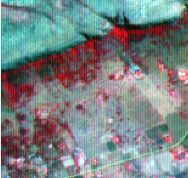
Close-up of a color display of three bands of a raw ASTER Level 1A image. Red = Band 3 (near-infrared), Green = Band 2 (red), Blue = Band 1 (green). Prominent vertical striping is evident. For these wavelength bands, all image values in a horizontal line of cells are acquired simultaneously by a linear array of detectors. Each vertical column represents the sequential output of a single detector, and differences in calibration between adjacent detectors give rise to the striping.
