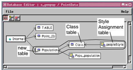
The relationships between the three tables required for stalk or root display by attribute using the color stack feature are circled in the Database Editor at the right.
