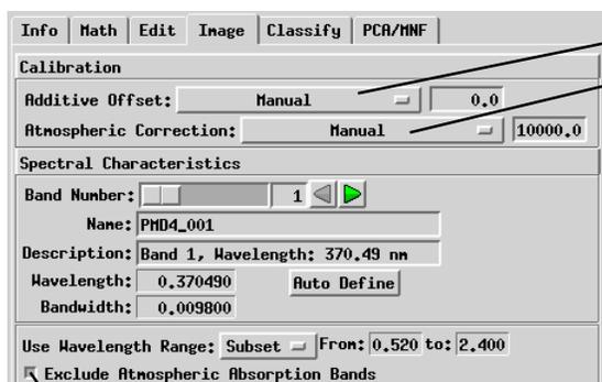
You can now automatically exclude from processing the two ranges of spectral bands near 1.4 and 1.9  $\mu\text{m}$  that are severely degraded by water vapor absorption. These ranges are shown as gaps in spectral plots, as in the plot to the right.
