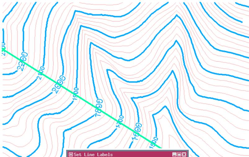
A new tool has been incorporated into the Spatial Data Editor to place labels on lines that intersect the segment you draw for label positioning. You can designate the orientation of the label relative to the tool or the object and also indicate whether it should be above, below, or centered on the line. There is even an “assistant” to help you write your label style query.
