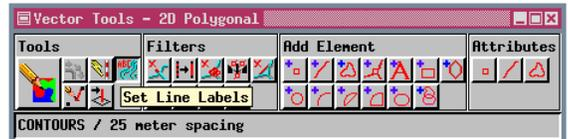
This query sets label styles (size, color, and position) for contour lines. Styles vary such that large labels appear on contours with z-values evenly divisible by 200.
