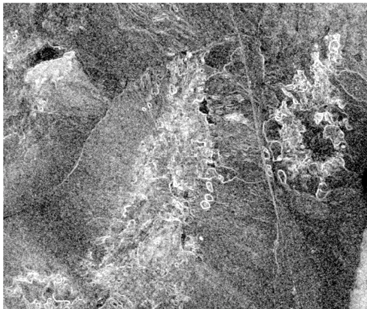
Figure 10. Sample results from the Auto-Correlogram process for the 1997 AVIRIS scene of Cuprite, using the 1.98 to 2.467 mm band subset. Pixel gray levels represent the average spectral angle between each pixel and its adjacent neighbors (with contrast stretch applied). Spectrally uniform areas appear dark, while bright pixels separate areas with contrasting spectral characteristics.
