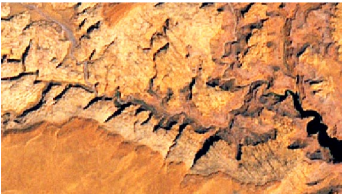
Left, color satellite image (15-m cell size) of desert area with exposed rock layers exhibiting northwest-trending vertical fractures. Right, same image displayed with integrated filtering
