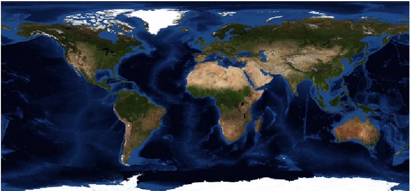
NASA Blue Marble global image (43,200 lines by 86,400 columns, 460-meter cell size) exported to BigTIFF. File size is 10.4 GB uncompressed or 4.08 GB with lossless LZW compression.
