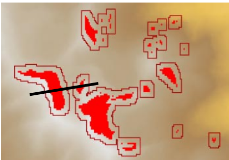
Brown lines outline a 3-cell buffer zone used in this example for feathering the edges of void fills.
