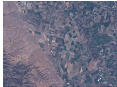
SRFI Option 1: Scaled reflectance at top of atmosphere. Atmospheric haze and attenuation remain and affect the overall image brightness. Band-by-band differences in these effects also alter the color-balance of these RGB images.
