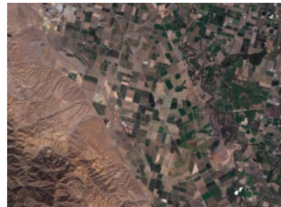
SRFI Option 3: Scaled reflectance of Earth surface materials with all atmospheric effects (path reflectance and atmospheric attenuation) removed. Remaining brightness variations due to varying slope angles and directions in hilly areas can be corrected using the TERCOR geospatial script (see the color plate entitled Scripts by Jack: Correct for Terrain Induced Radiance Effects ).
