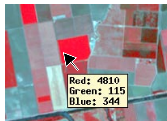
SRFI Option 3: Scaled reflectance of Earth surface materials with all atmospheric effects (path reflectance and atmospheric attenuation) removed. Remaining brightness variations due to varying slope angles and directions in hilly areas can be corrected using the TERCOR geospatial script (see the color plate entitled Scripts by Jack: Correct for Terrain Induced Radiance Effects ).
