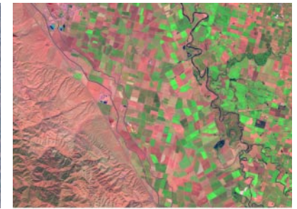
SRFI Option 1: Scaled reflectance at top of atmosphere. Atmospheric haze and attenuation remain and affect the overall image brightness. Band-by-band differences in these effects also alter the color-balance of these RGB images.
