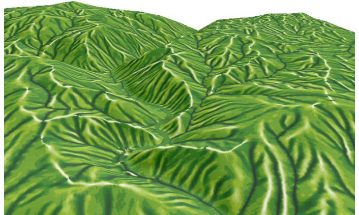
Plan (contour) curvature raster produced by the SURFCURVE script, displayed with color palette over the terrain. Positive values indicate convex-outward surfaces.
