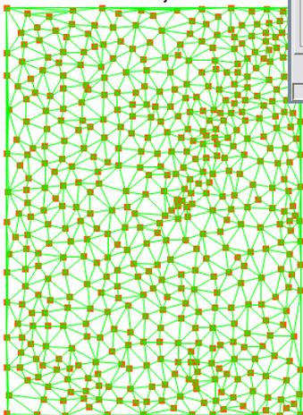
You have worked with TINs as input objects in previous exercises. To create a TIN object, use the Triangulation operation. **Triangulation** computes a TIN from points in a vector or database object, from vector contours, or from a raster object.
