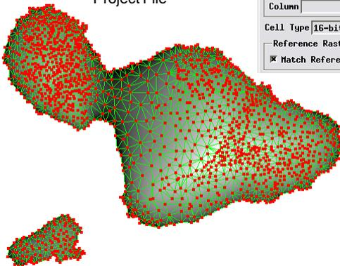
When the input TIN object has more than one hull, Triangle Interpolation produces a separate elevation surface for each hull, with intervening cells marked as null.
