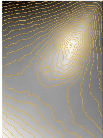
You can smooth the contour lines produced by this and other contouring methods using the Vector Filters process (Geometric Filter from the TNTmips menu). The Line Densification filter adds vertices to lines to make them better approximate a smooth curve. You can find more information about Line Densification in the *Advanced Vector Editing and Digitizing Soil Maps* tutorials.
