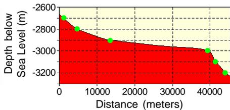
Detail of computed surface from previous page (left) and this page (right) with profiles along the green line. Green dots on profiles mark points where profile crosses input contour lines; arrows on left profile mark crossings of nonexistent contours due to unconstrained oscillations of the minimum curvature surface between widely-spaced contours. Increasing the Coarse Grid Ratio and Tension values helps damp these extraneous oscillations.
