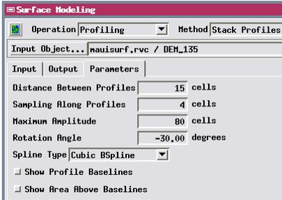
If profiles appear “noisy” (too detailed), you can either increase the value of the Sampling Along Profile parameter or smooth the profile. The profile is smoothed by splining, with a choice of either Cubic (third order) B Spline, or Quadratic (second order) B Spline methods.
