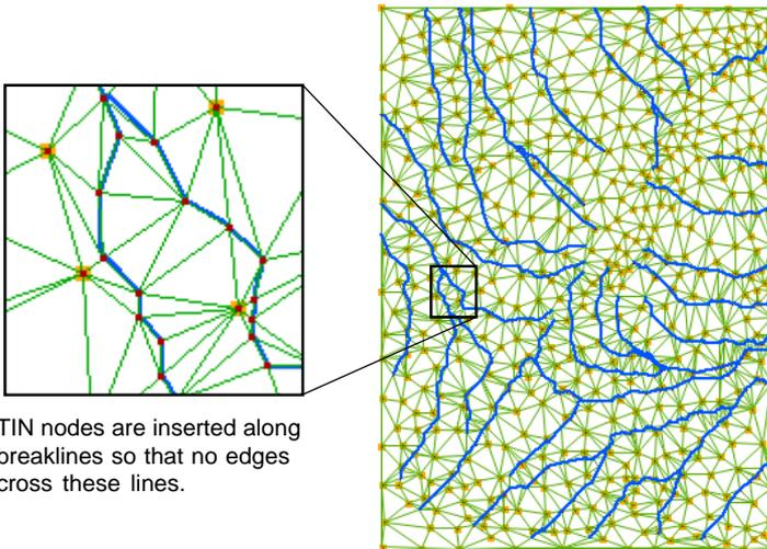
TIN nodes are inserted along breaklines so that no edges cross these lines.
