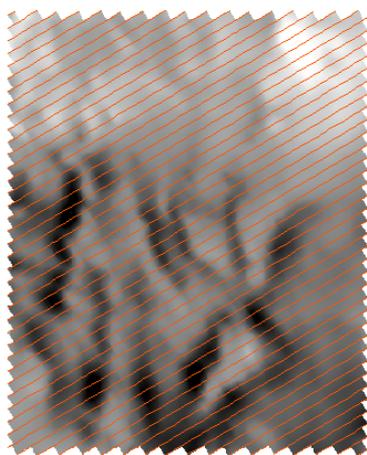
These transect lines are from an aeromagnetic survey of a single 7.5-minute map quadrangle, with magnetic intensity values in nanoteslas.
