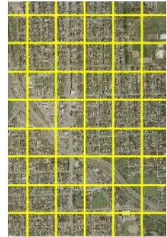
Portion of a color orthophoto overlaid with a map grid with 200 meter spacing between the grid lines.
