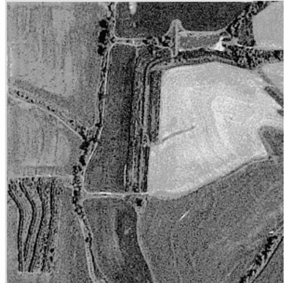
Same image with 5 x 5 High Pass filter applied (auto-normalized contrast). The image appears sharper, with clearer edges and enhanced details.
