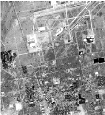
Upper right part of raster object TM3NOISY (input image), which shows horizontal striping.
