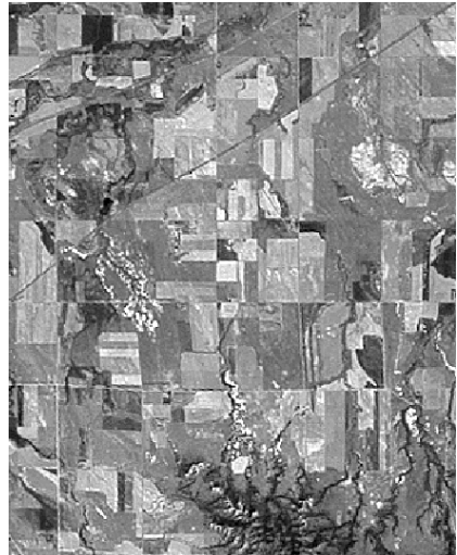
Same image area with 3 x 3 Volterra / Unsharp filter applied (displayed with auto-linear contrast), providing significant enhancement of edges and line features.
