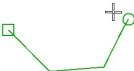
When the cursor is the crosshairs shape, it adds to the end of the line unless it is within the snap distance of the start (in which case it adds to the start).
